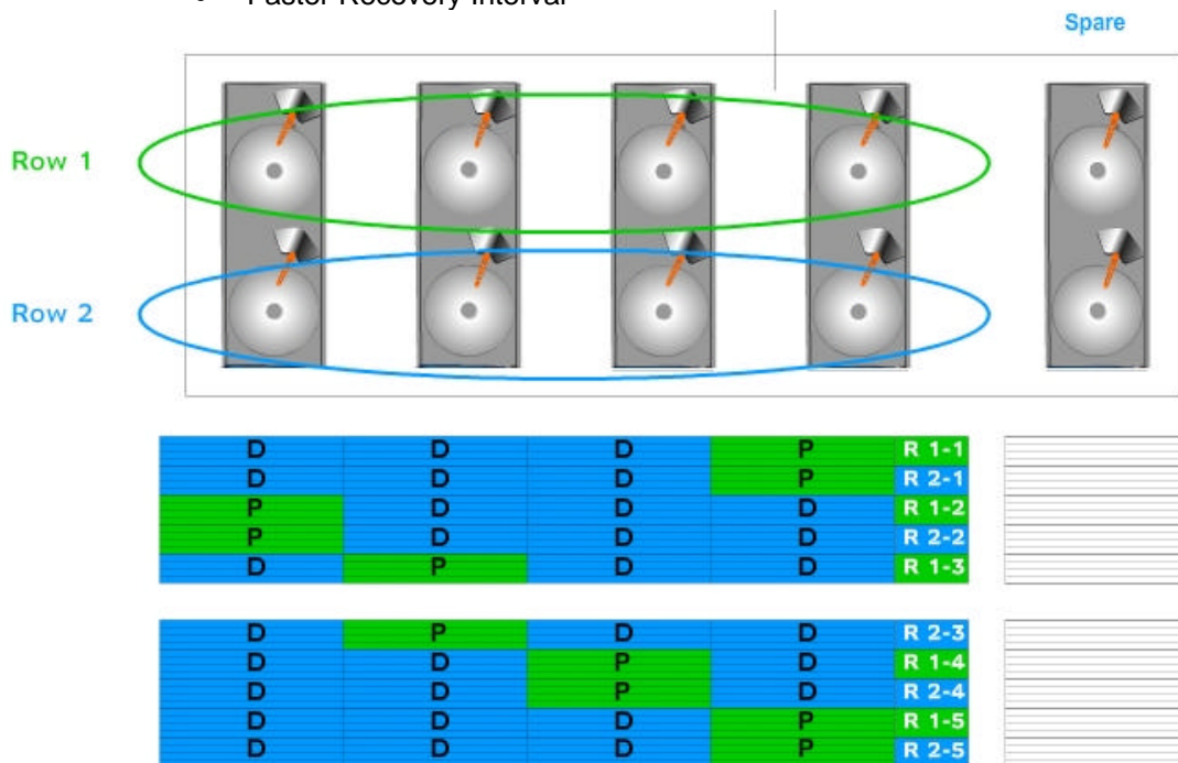
RAID 50 Interleaved Set in Dual Drive HD Enclosure with Spares Available
